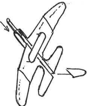
Sketch design on to 3x5 card Including all parts, tabs, etc Cut, fold, trim symmetrical parts Cut other parts Gluestick tape body sides/tabs Fold crease wing dihedral/camber Clay or toothpick for nose weight Fly. Enjoy. Repeat.
