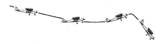
When the nose drops, the plane will gain some speed. Give it a little more power as you gently give the plane up elevator to bring the plane nose level with the horizon.
