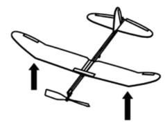
Pilots of full-scale airplanes as well as model aircraft must correctly determine the CG before flight to ensure that the airplane is balanced.
